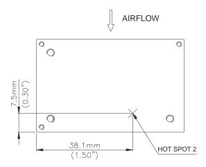
**Figure 15:** \* Hot spot 2 temperature measured point, the allowed maximum hot spot 2 temperature is defined at 108  $^{\circ}$ C
