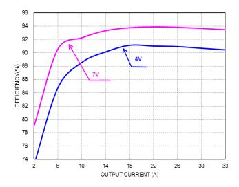
**Figure 1:** Efficiency vs. load current for 7V\_Vout, 4V\_Vout at 54V input voltage at 25°C.
