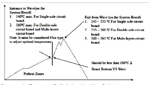
Recommended Temperature Profile for Lead-free Wave Soldering
