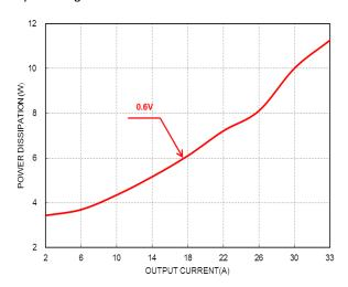
**Figure 4:** Power loss vs. load current for 0.6V\_Vout at 54V input voltage at 25°C.
