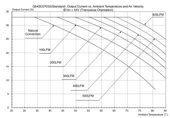
**Figure 14:** Output current vs. ambient temperature and air velocity @Vin=54V(Transverse Orientation, airflow from Vin+to Vin-, without heat spreader)
