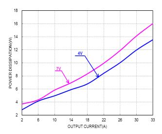
**Figure 2:** Power loss vs. load current for 7V\_Vout,4V\_Vout at 54V input voltage at 25°C.
