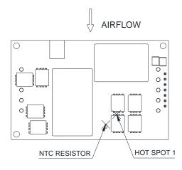
**Figure 13:** \* Hot spot 1& NTC resistor temperature measured point, the allowed maximum hot spot 1 temperature is defined at 118  $^{\circ}$
