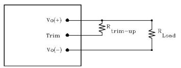
Figure 10: Circuit configuration for trim-up (increase output voltage)
