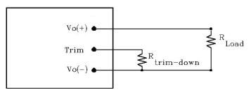
Figure 9: Circuit configuration for trim-down (decrease output voltage)
