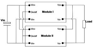
Figure 11: Parallel and droop current sharing configuration for no redundancy requirement system
