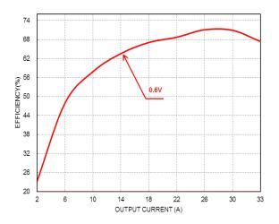
**Figure 3:** Efficiency vs. load current for 0.6V\_Vout at 54V input voltage at 25°C.
