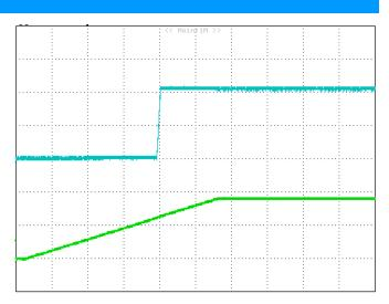
**Figure 6:**Turn-on transient at zero load current (100 ms/div). Top Trace: Vout; 2V/div; Bottom Trace: input voltage: 20V/div.
