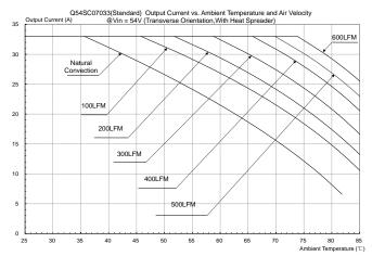
**Figure 16:** Output current vs. ambient temperature and air velocity @Vin=54V(Transverse Orientation, airflow from Vin+ to Vin-,with heat spreader)
