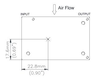
**Figure 16:** Hot spot 1 temperature measurement location The allowed maximum hot spot 1 temperature is defined at  $112\,^{\circ}C$ .
