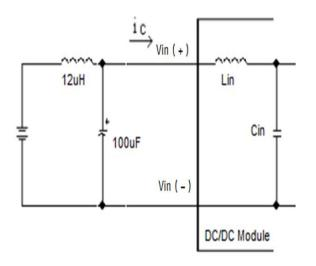
Figure 8: Test Setup Diagram for Input Ripple Current Note: Measured input reflected-ripple current with a simulated source Inductance of 12µH. Measure current as shown above.
