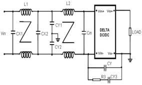
Figure 12-1: Recommended Input Filter
