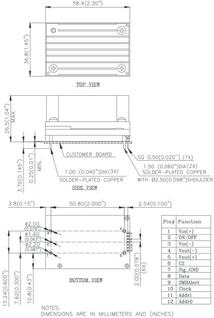
DIMENSIONS ARE IN MILLIMETERS AND (INCHES)
