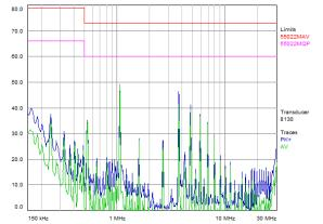
Figure 12-2: Test Result of EMC (Vin=54V, Io=51A).
