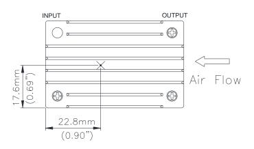
**Figure 18:** Hot spot 2 temperature measurement location The allowed maximum hot spot 2 temperature is defined at 110  $^{\circ}$ C.
