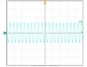
**Figure 11: Output Voltage Ripple and Noise** at nominal input voltage and max load current (20 mV/div, 2us/div) Load cap: 660uF (100uF MLCC+560uF Oscon).
